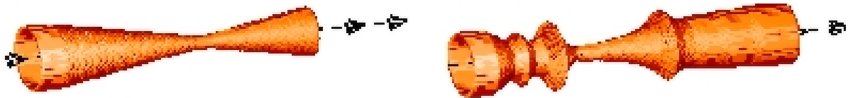
Figure 1: Optimization of a nozzle for a two-phase flow with an ES. No simulation model was available at the time [Sch68]. Schwefel performed an experimental optimization using an (1+1) ES. The nozzles were built of conical pieces such that no discontinuity within the internal shape was possible. In this way every nozzle shape could be represented by its overall length and the inside diameters at the borders between the segments (every 10mm). Despite the use of a very simple (1+1) ES without recombination this first ES using gene duplication and deletion produced astonishingly good results leading to a ‘strange’ nozzle shape shown on the right. The unintuitively formed shape has been understood only after further investigations. On the left, the starting shape is shown.
