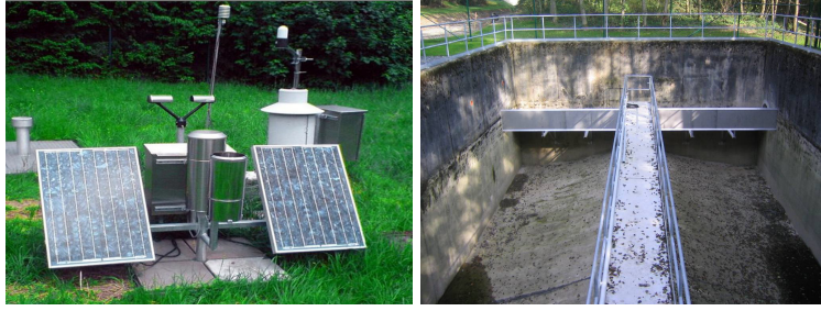
Fig. 1: Left: rain gauge (pluviometer). Right: stormwater tank.
