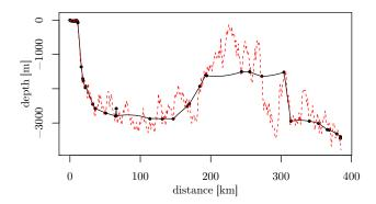
Figure 1: Undersea cable depth estimation (black line) and conditional simulation (dashed red line) and the given data (black dots). Based on the example presented in [18].
